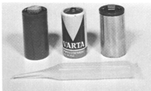
Figure 2. View of two liquid fuel air cells and of a D-size dry cell
