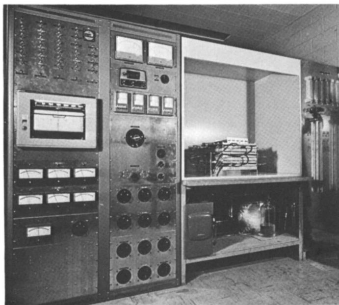
Figure 6. Test station with 500-watt matrix fuel cell battery
